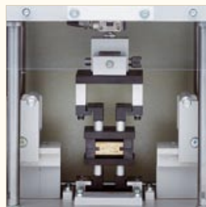
Internal bond strength of grooved sample strips (quick alternative method)
