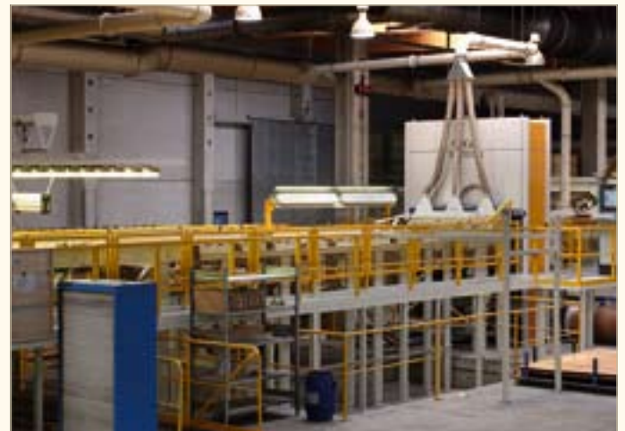
Laminat flooring inspection (one-sided)
