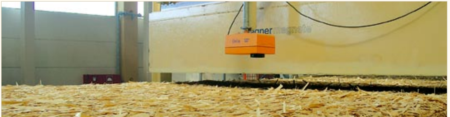
Moisture measurement after the forming line
